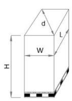
The depth (L) of the package is limited to 2000 mm for a better management of transport line, also if theoretically has no limits. The strapping product has the following maximum measures, according to the machine, while the minimum dimensions of W and L are 500, instead of H that is 600 mm. In case of package turning, the maximum diagonal (d) allowed, assume the same value of W max.
