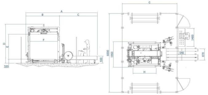
The dimensional drawing refers to the version with lance, decoiler and electric panel on the right, but they can be positioned in both sides. The SIZE table indicates the standard widths of the machine, the MODEL table indicates the heights.
