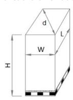
The depth (L) of the package is limited to 2000 mm for a better management of transport line, also if theoretically has no limits. The strapping product has the following maximum measures, according to the machine, while the minimum dimensions of W and L are 500, instead of H that is 600 mm. In case of package turning, the maximum diagonal (d) allowed, assume the same value of W max.
