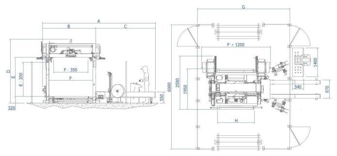
The dimensional drawing refers to the version with lance, decoiler and electric panel on the right, but they can be positioned in both sides. The SIZE table indicates the standard widths of the machine, the MODEL table indicates the heights.
