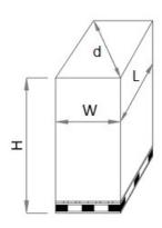
The depth (L) of the package is limited to 2000 mm for a better management of transport line, also if theoretically has no limits. The strapping product has the following maximum measures, according to the machine, while all the minimum dimensions are 500 mm. In case of package turning, the maximum diagonal (d) allowed, assume the same value of W max.
