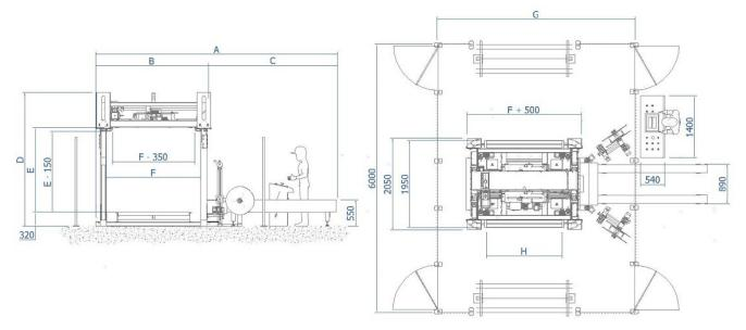
The dimensional drawing refers to the version with lance, decoiler and electric panel on the right, but they can be positioned in both sides.
