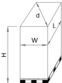
The depth (L) of the package is limited to 2000 mm for a better management of transport line, also if theoretically has no limits. The strapping product has the following maximum measures, according to the machine, while all the minimum dimensions are 500 mm. In case of package turning, the maximum diagonal (d) allowed, assume the same value of W max.
