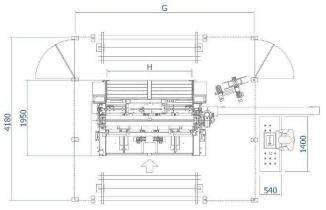
The dimensional drawing refers to the version with lance, decoiler and electric panel on the right, but they can be positioned in both sides. The SIZE table indicates the standard widths of the machine, the MODEL table indicates the heights.
