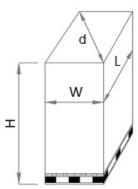
The depth (L) of the package is limited to 2000 mm for a better management of transport line, also if theoretically has no limits. The strapping product has the following maximum measures, according to the machine, while all the minimum dimensions are 500 mm.
