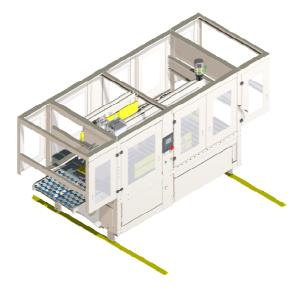
The one head PRIMA jogger model PM1 is a fully automatic machine, which, after selecting the strapping program (0 or 1), is activated and does not require the intervention of any operator.
