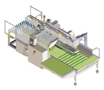
The PC3 "Compact" jogger is a fully automatic machine which, after selecting the strapping program (0, 1 or 2), is activated and does not require the intervention of any operator. It was manufactured to square and strap transversally packages of corrugated cardboard boxes. It combines the most up-to-date control and safety technologies in its sector with a robust, solid and long-lasting mechanical structure.
